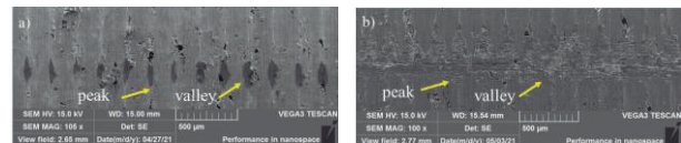
Figure 2 Morphology of wear marks for (a) surface with wear less than 4 \times 10^{-6} \text{ mm}^3 \cdot \text{N}^{-1} \cdot \text{m}^{-1} and (b) surface with wear more than 4 \times 10^{-6} \text{ mm}^3 \cdot \text{N}^{-1} \cdot \text{m}^{-1} .
