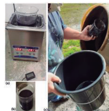
Figure 2 Dispersion of the nanosheets: (a) ultrasound; (b) dispersion in water; (c) mixing of the dispersion into the concrete.
