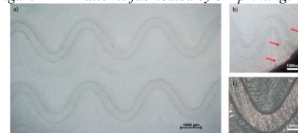
Figure 3 Patterns fabricated by micro-CNC.
