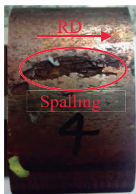
Figure 1 Top of rail showing a spalling.
