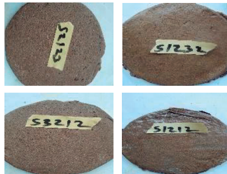
Figure 3 Developed brakepad materials samples after curing
