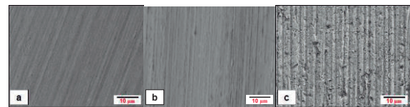
Figure 3 SEM images in the centre of wear scar on AISI 304 samples after the micro-abrasion-corrosion tests with different counter-bodies : (a) PP; (b) POM; (c) Si 3 N 4 .
